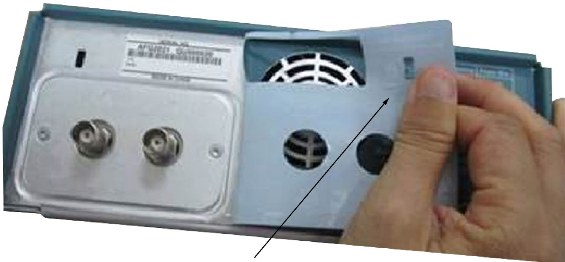
Figure 24: Peeling off the rear panel label
