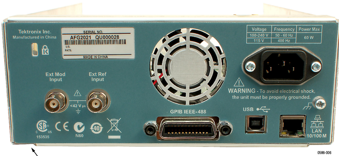
Figure 23: Location to start removing the rear panel label
