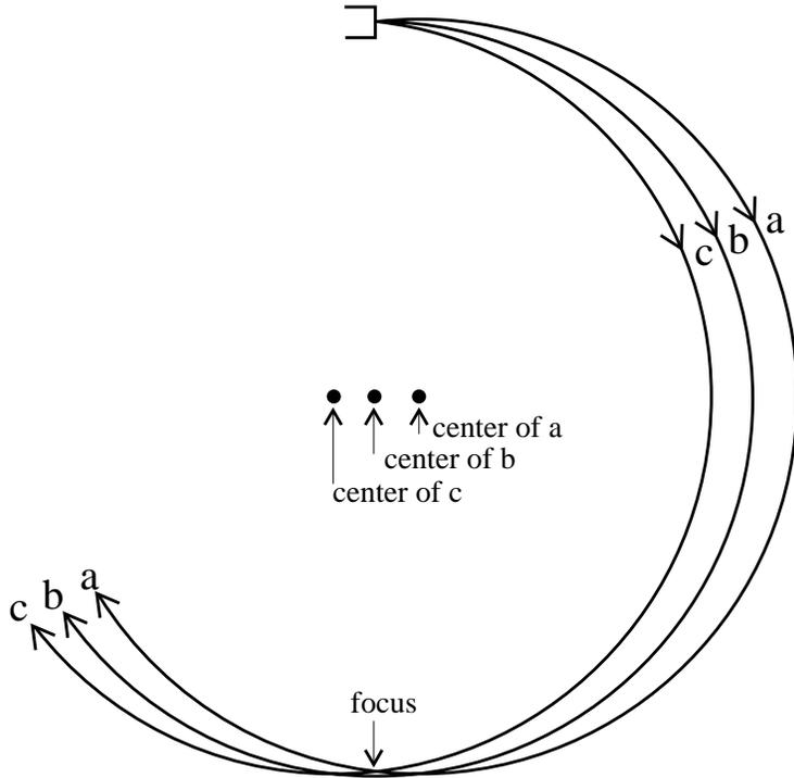
Note that the particles will pass through a focus point one diameter away from the source. Of course, if the angles are very large then the particle will pass near the focus. You may like to show that the particle will miss the focus by a distance  $\epsilon$ .
