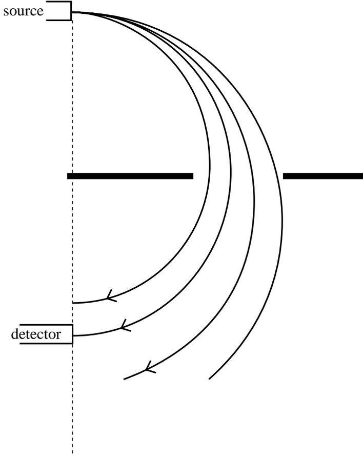
The particles of different momenta will pass through different focus points. By using a small source and a small detector only those in a small range from  $p$  to  $p + dp$  will be accepted.
