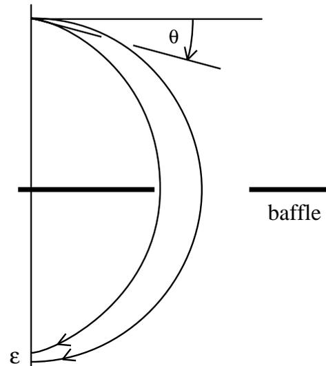
Because  $\sin^2 \theta$  changes slowly near  $\theta = 0$ ,  $\epsilon$  is very small. A baffle with a slit is used to restrict the detected particles to those with  $\theta$  small. In this spectrometer the restriction is:
