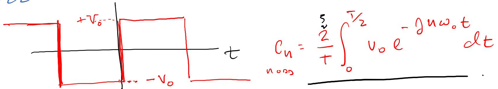
$$c_n = \frac{2}{T} \int_0^{T/2} V_0 e^{-jn\omega_0 t} dt$$
