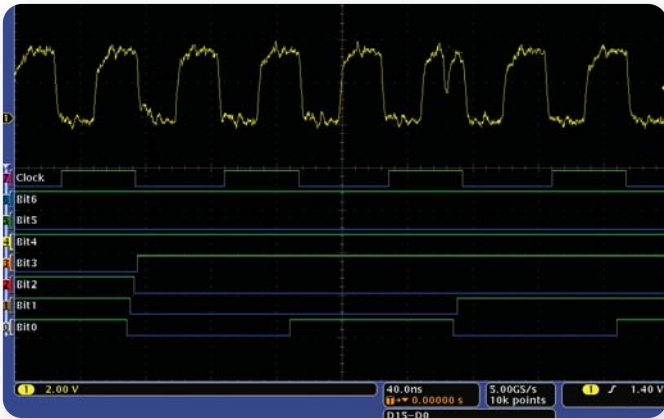
► Figure 7. Analog and digital waveforms acquired with a single instrument - The MSO4000 Series.
