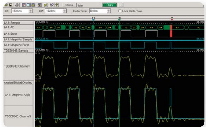
▶ Figure 5. Timing analysis using a Tektronix TLA Logic Analyzer.
