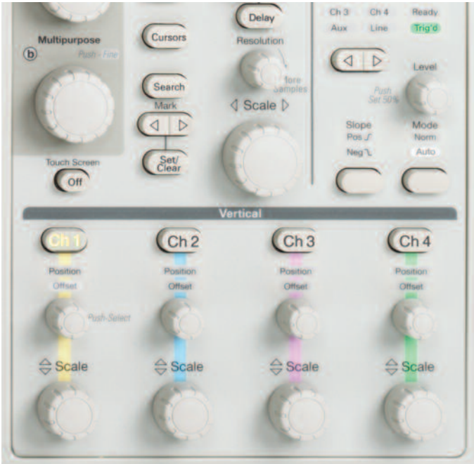
Figure 60. Traditional, analog-style knobs control position, scale, intensity, etc. — precisely as you would expect.
