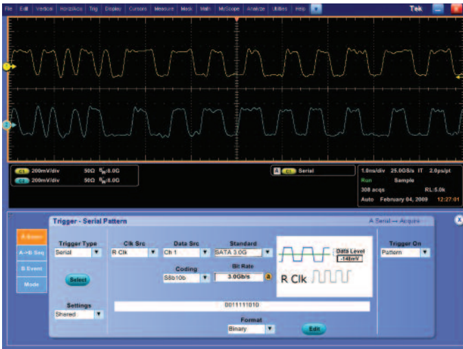
Figure 51. A DPO provides an ideal solution for non-repetitive, high-speed, multi-channel digital design applications.
