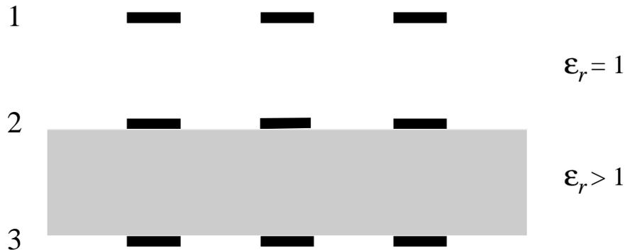
The capacitance between electrode sets 2 and 3 is  $\epsilon_r$  times larger than between sets 1 and 2.
