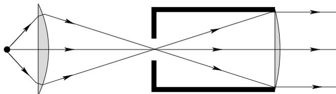
thru the collimator thereby facilitating detection of weak spectral lines. For strong lines it permits narrowing the slit width and thus improving resolution. Use such a lens (mounted on a ring stand) to find an arrangement which fills the collimator with light.
