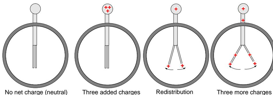
Figure 1: *Qualitative* schematic of electroscope response.
