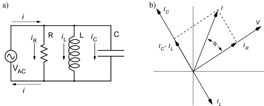
Figure 3: A parallel LRC circuit.
