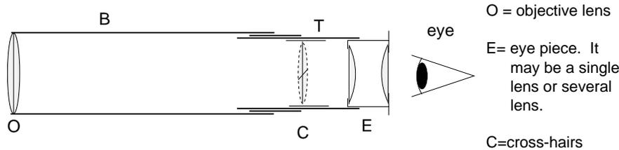
The eyepiece E slides back and forth in the tube T and one should first adjust the eyepiece to give a clear image of the cross hairs. Then move the tube T back and forth in the barrel B until the image of a distant object, formed by the objective O, falls on the plane of the cross hairs. The test for this is the absence of parallax between the cross hairs and image.
