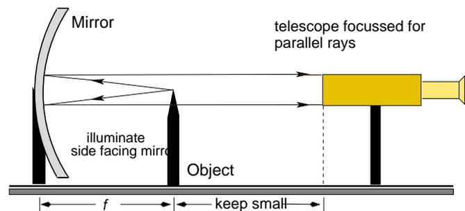
**Figure 3:** Object at  $f$ , image at infinity.
