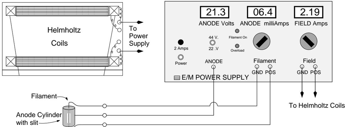
Figure 5: Basic wiring layout.
