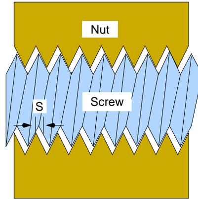
Figure 1: Backlash in screw mechanism.
