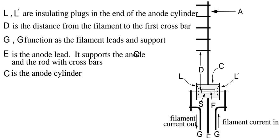
If the tube is properly oriented, the velocity of the emerging electrons is perpendicular to the magnetic field. Hence the magnetic force vector  $\vec{F}$ , which is described as a cross product  $\vec{F} = e(\vec{v} \times \vec{B})$ , supplies the centripetal force  $\frac{mv^2}{r}$  for a circular path of radius  $r$ . Since  $\vec{v}$  is perpendicular to  $\vec{B}$
