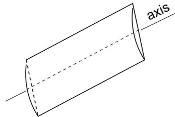
Figure 2: Cylindrical lens.
