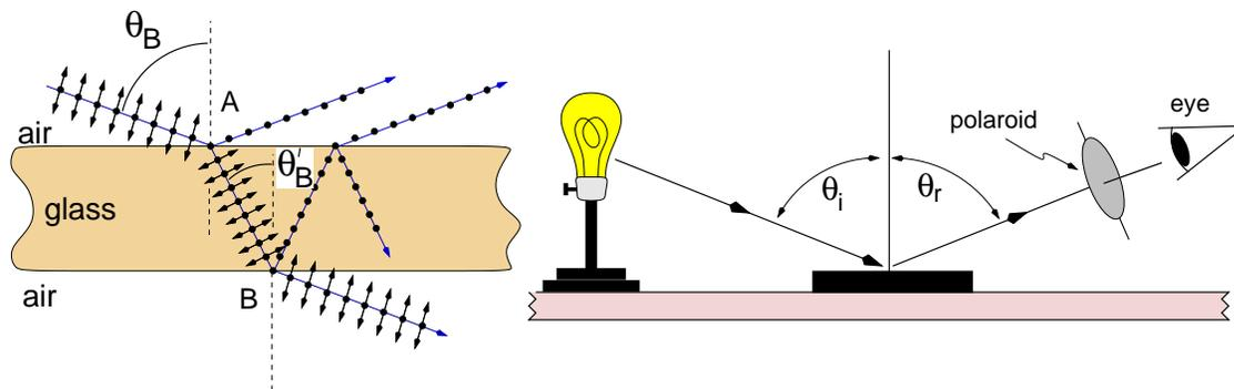
Figure 1: Reflection and transmission of light at Brewster's angle.
