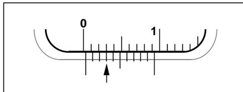
Figure 2: The vernier reads  $0.03\text{ cm}$
