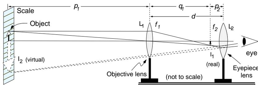
Figure 1: The inverting telescope (not drawn to scale).
