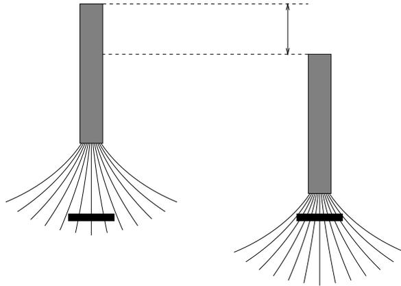
Figure 3: A moving magnet - lines move across a wire
