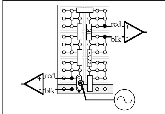
Figure 8: Inputs to differential amplifiers.
