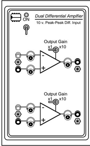
Figure 7: Dual differential amplifier module.
