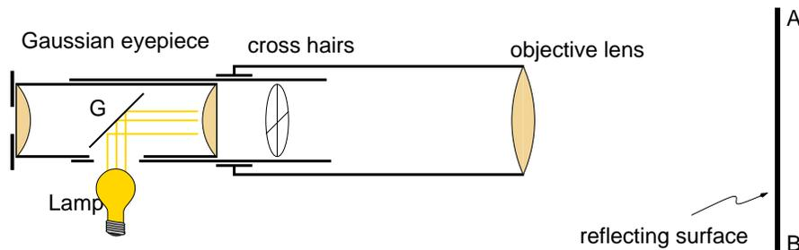
Figure 4: Spectrometer telescope
