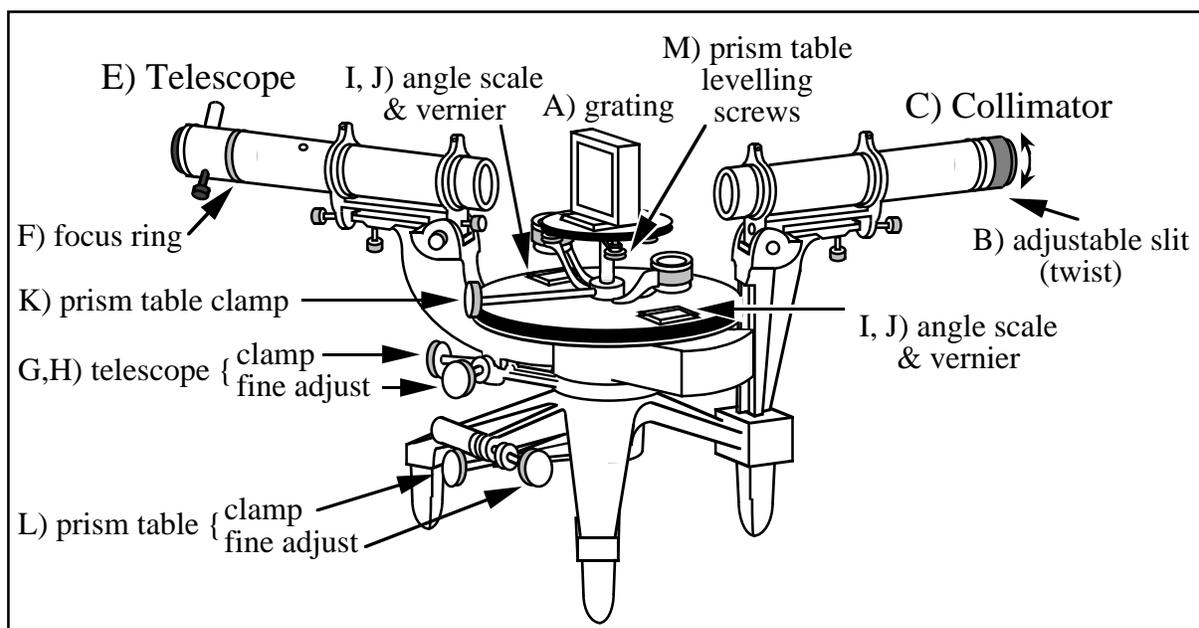
Figure 1: The spectrometer (side view).
