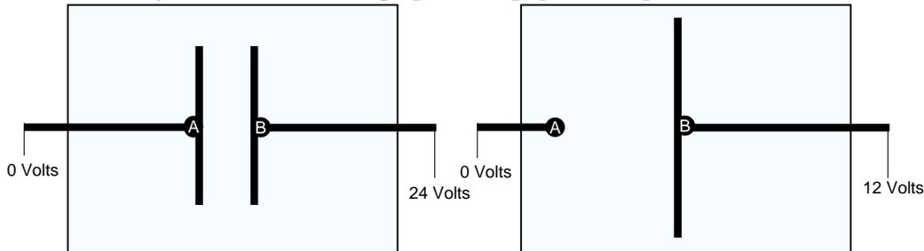
Figure 3: Electrode configurations for (a) parallel plates (left) and (b) "half" dipole (right).
