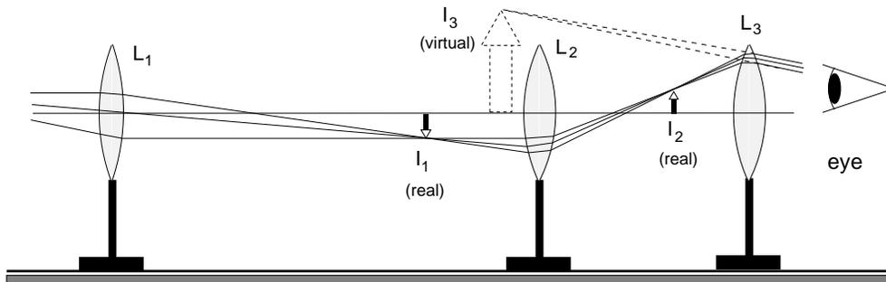
Figure 4: Configuration of a three lens erecting telescope.
