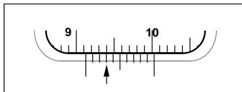
Figure 3: The vernier reads  $9.13\text{ cm}$
