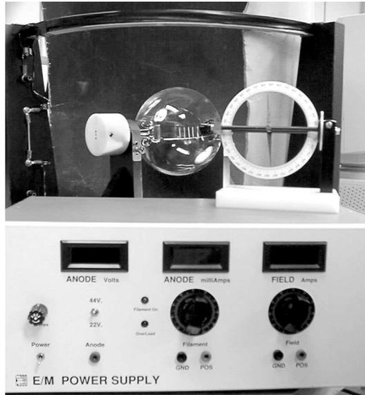
Figure 1: Foreground: dip-needle magnetic-field sensor sitting on power supplies with built-in digital meters; Background: Sargent-Welch  $e/m$  equipment and black cardboard.
