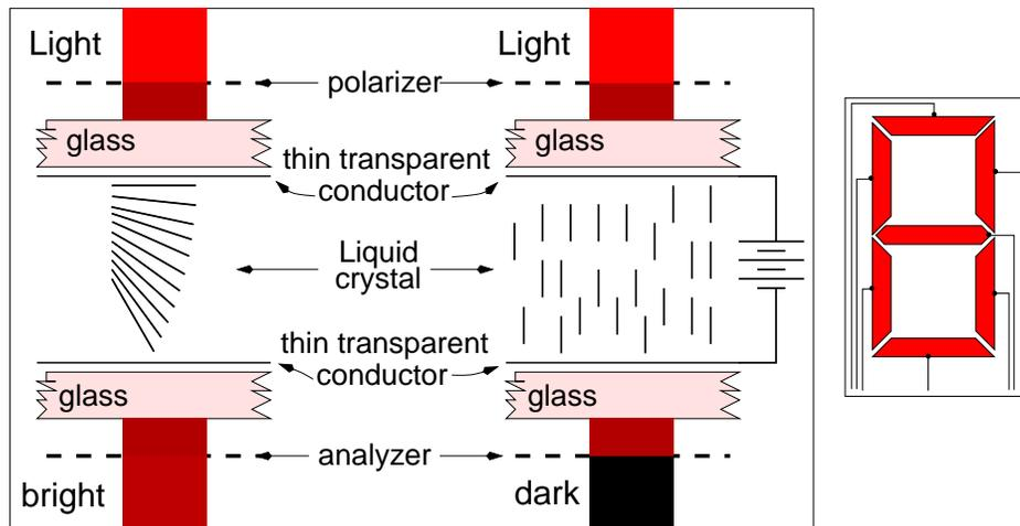
Figure 3: Construction of a liquid crystal display
