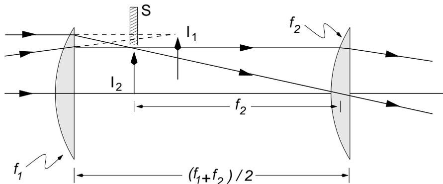
Figure 7: Construction of a Huygens eyepiece.
