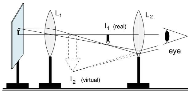
Figure 5: Setup for compound microscope.
