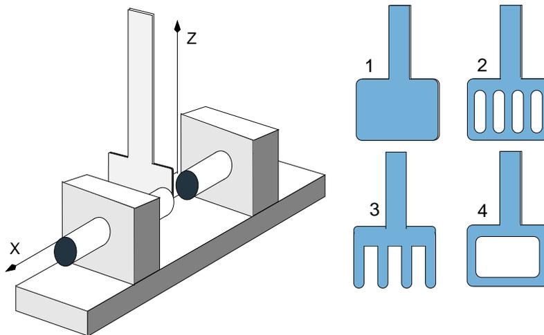
Figure 1: The magnet and the paddle pendulum.
