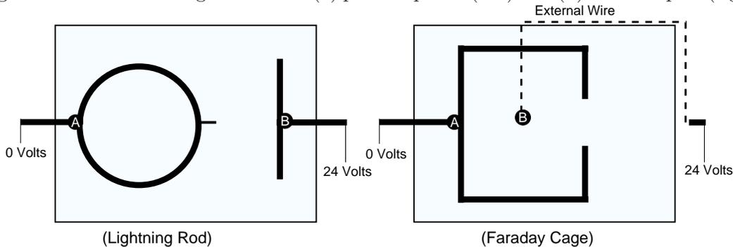
Figure 4: Two other electrode configurations, (a) lightning rod, (b) Faraday Cage.
