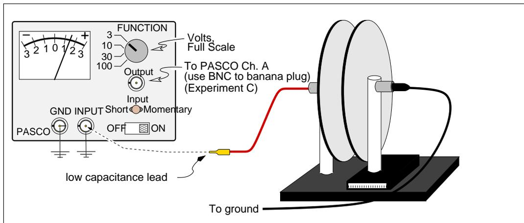
Figure 1b: Reading the voltage
