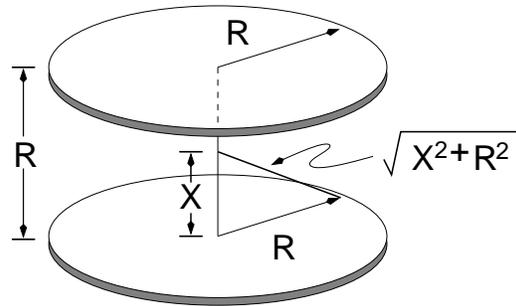
Figure 4: Helmholtz coil geometry.
