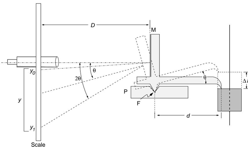
Figure 1: Schematic of the optical lever.
