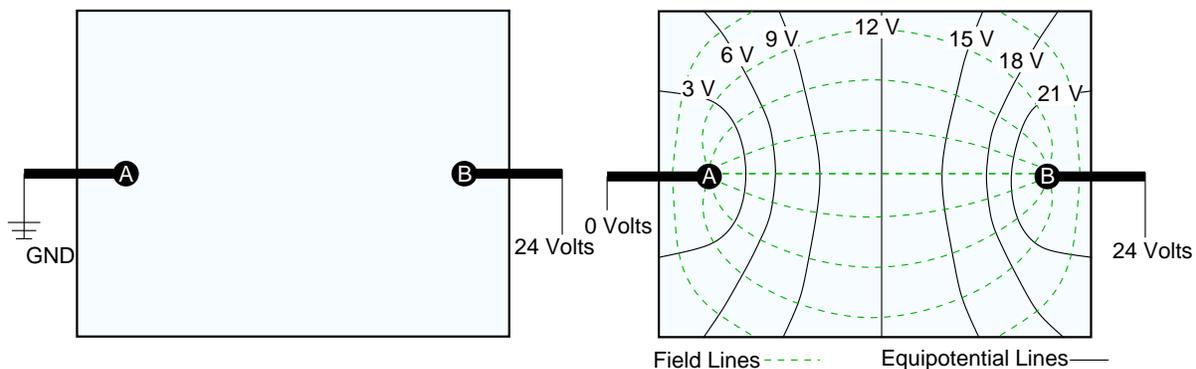
Figure 2: Electrode placement that qualitatively approximates a charge dipole configuration.
