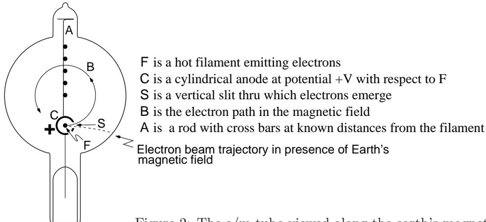
Figure 2: The e/m tube viewed along the earth's magnetic field (i.e.,  $B_{\text{earth}}$  is perpendicular to the page).
