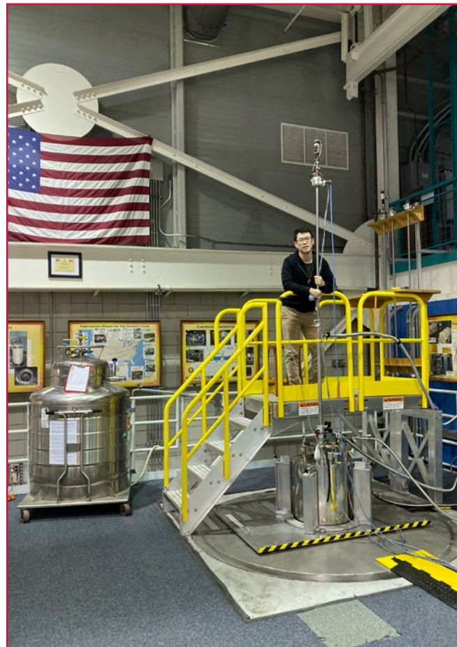
Tiancheng Song is doing an experiment using the 45 Tesla Hybrid Magnet, which produces the highest DC magnetic field in the world.
